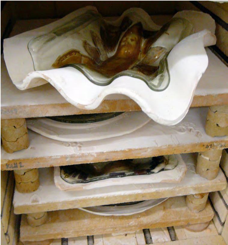
7 Slumped glass pieces and their molds
