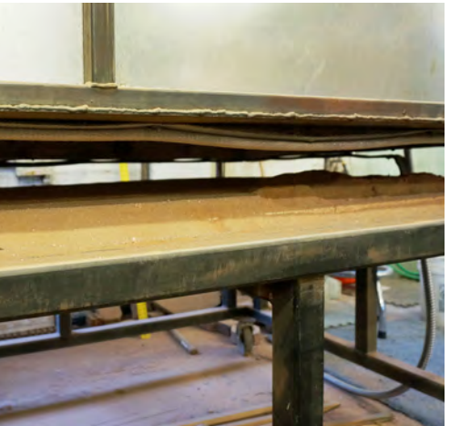
9 Sand bed and kiln. The pattern is pressed into the sand bed, deforming the sand into the shape of the pattern. The sheet of glass is carefully placed onto the sand, and then the kiln is closed for heating
