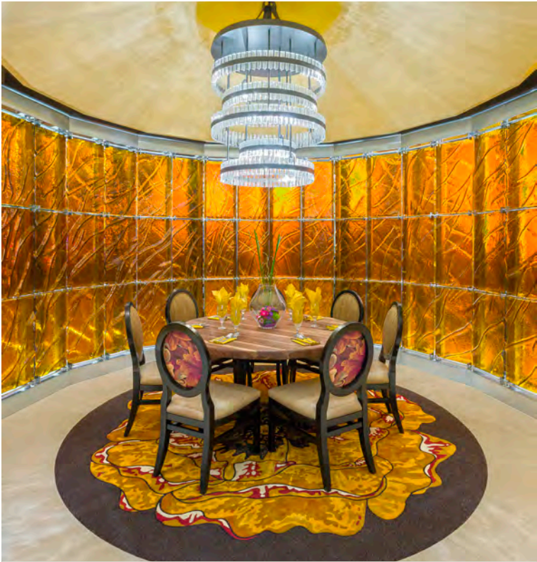
4 Laurel Porcari, architectural art glass in The Beacon , a private dining room in L'Auberge Casino and Hotel , Baton Rouge, Louisiana. Made with fused art glass, slumped on a plaster mold and a custom stainless steel armature
