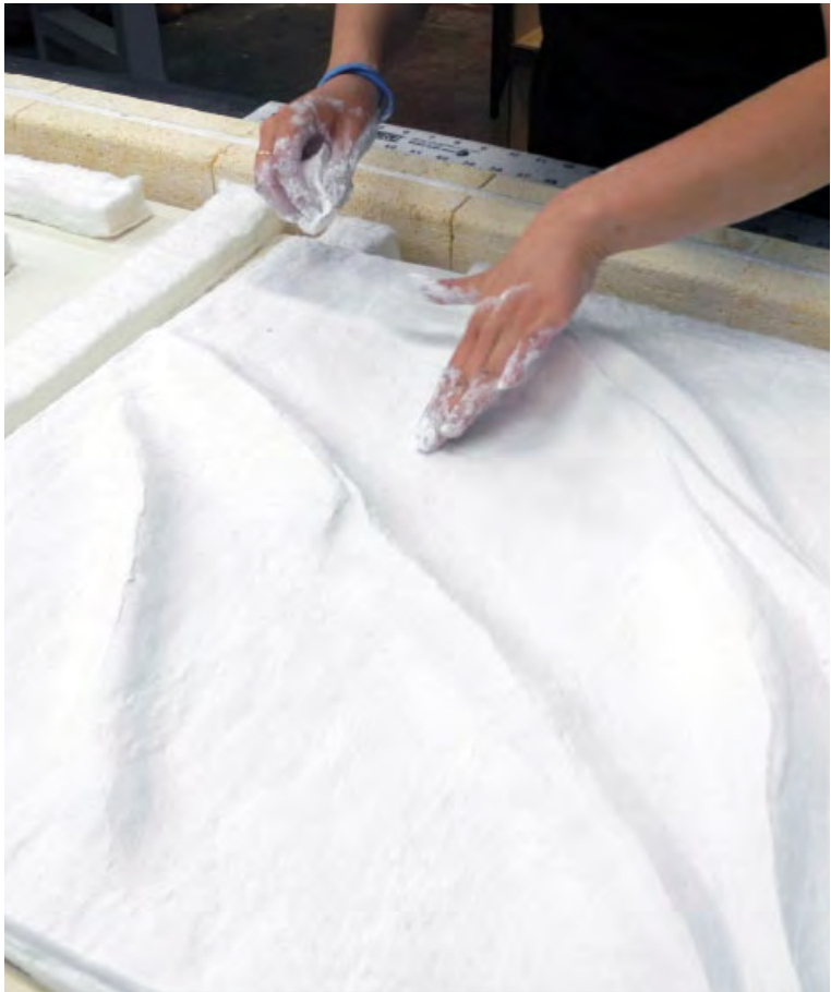
6 Laurel Porcari shaping the plaster mold to be used in the kiln
